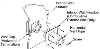
Figure 27 - Connecting Vent Cap with Horizontal Vent Pipe
